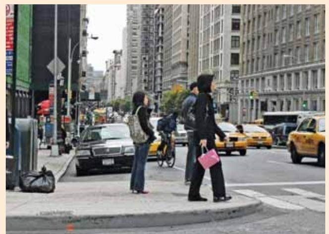
The curb extension on the southeast corner shortens the crossing distances and aligns the curbs to make for a safer crossing.
