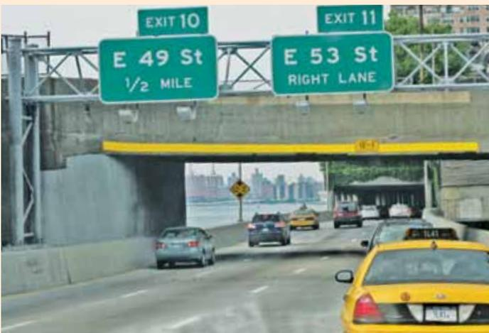
Bridge strikes at the E. 60<sup>th</sup>/ 61<sup>st</sup> Street overpass on the FDR Drive are down 56% since the treatment was installed, the greatest reduction of any pilot location.
